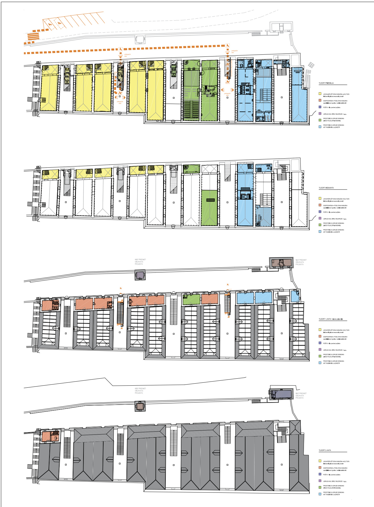
Fig. 8. Reconstruction project, new function of the Lazaretto space, scale 1:200. From: Architectural-construction project of the Lazaretto reconstruction - Dubrovnik. Amendments to the main project, December 2011.
